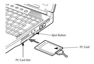
Figure 4-8 Installing/Removing PC Cards
